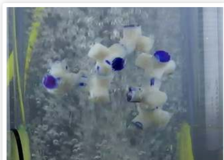
Figure 8: photograph of an experiment in which many tetrapods were entered into the system. In this case the tetrapods organize into 2 separate chains. The particles are being agitated by the flow of air bubbles in the surrounding medium.
